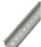
DIN rail perforated, Standard profile, width: 35 mm, height: 7.5 mm, acc. to EN 60715, material: Steel, galvanized, passivated with a thick layer, length: 2000 mm, color: silver
