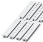
Zack marker strip, Strip, white, labeled, can be labeled with: CMS-P1-PLOTTER, printed horizontally: consecutive numbers 1 ... 10, 11 ... 20, etc. up to 91 ... 100, mounting type: snap into tall marker groove, for terminal block width: 8.2 mm, lettering field size: 10.5 x 8.15 mm, Number of individual labels: 10
