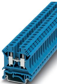
Feed-through terminal block, nom. voltage: 800 V, nominal current: 41 A, connection method: Screw connection, number of connections: 2, cross section: 0.2 mm<sup>2</sup> - 10 mm<sup>2</sup>, AWG: 24 - 8, width: 8.2 mm, color: blue, mounting type: NS 35/7,5, NS 35/15
